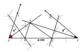
Construction of  $\triangle ABC$ , given the perimeter (AB + BC + CA) = 'a' cm,  $\angle B = x^{\circ}$  and  $\angle C = y^{\circ}$ .
